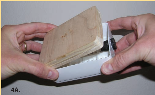
Figure 4A. The pipet tip box is placed over a piece of \frac{3}{4} " plywood cut to size. 4B. It is secured in place with hot glue.
